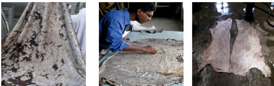
Figure 4: Enzyme only leather dehairing using alkaline protease IMTECH 04 was carried out in collaboration with Central Leather Research Institute (CLRI), Chennai.
